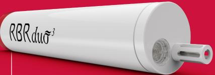
The RBR*duo*<sup>3</sup> instruments can integrate almost any two sensors from RBR, offering high accuracy, flexible schedules, USB-C download, Wi-Fi communication, and twist activation. Variants with pressure, temperature, conductivity, radiometer, PAR, and turbidity sensors are also available in titanium housing for deep applications (| deep), designed to endure harsh conditions.
